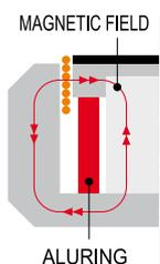
*For the mid-woofer cones we chose the Curv: a rigid, light and damped material, made with pure polypropylene extruded, woven and heat treated. Furthermore, we have equipped the magnetic circuit with Aluring: an aluminium short circuit ring that reduces the non-linearity, which affects all the commonly made magnet systems, increasing the voice coil controlled excursion capability.*
